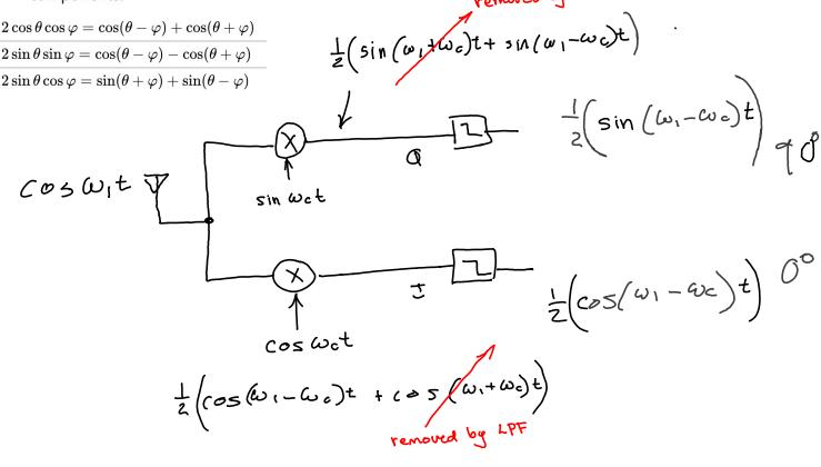
**Exercise 2**: What is the baseband spectrum if we add the I and Q branches above? What is the spectrum if the two branches have unequal gains? What if a DC offset is added to a mixer output?
