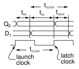
**Exercise 1:** Based on the diagram above, what is the setup time – the time from the input being valid to the latching clock edge?
