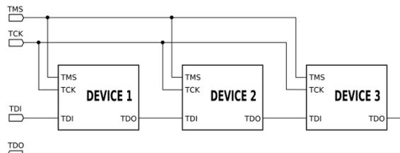
JTAG interfaces can also be used to program FPGAs, PLDs and various type of memory. They are also used to interface with on-chip debugging features such as logic analyzers, software debuggers, consoles and others.
