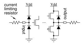
External clamp diodes can be used if the device does not include them or if they cannot handle the expected voltage or current levels. Schottky diodes can be used if a lower forward voltage drop (about 0.3 V) across the clamp diode is required.
