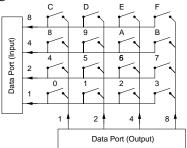
The digit or letter above each switch shows the label printed on the switch.
