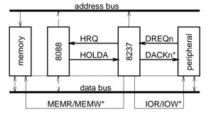
The DMA controller uses hold request (HRQ) and hold acknowledge (HOLDA) signals to ask the CPU to stop driving the address, data and control buses so that the DMA controller can drive them to carry out a transfer.
