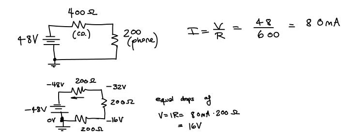
**Exercise 2**: If the battery voltage is 48V and the loop current is 48  $\mu$ A, what is the loop resistance? Is the phone on-hook or off-hook? What if the loop current is 48 mA?
