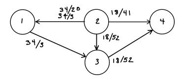
An ATM frame starting with the four header bytes 0x01 0x20 0x03 0x42 arrives at switch 2.
