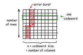
(d) To maximize the code rate, k/n, we want to make the codeword size, n, as large as possible. The codeword size, n, is also the interleaver width. Since the maximum interleaver size is 2048 the maximum codeword size is n = 2048/32 = $2^{11}/2^5 = 2^6 = 64$  bytes.
