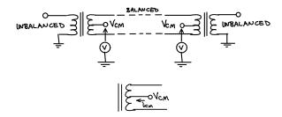
**Exercise 6:** If the common-mode circuit is used to carry 500mA, how much current flows through each half of the transformer secondary? What is the net effect on the flux in the transformer core?
