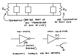
RS-485 is a standard similar to RS-422 that allows multiple drivers to be connected to a multi-drop bus. Only one device can have an active output at any given time – the others must be in a high-impedance mode.
