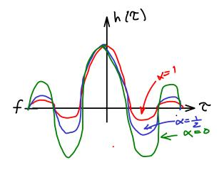
Larger values of excess bandwidth (wider bandwidth channels) results in less "ringing" of the impulse response which in turn reduces the amount of ISI near the sampling point of the next symbol. This makes the receiver less sensitive to errors in its timing of the sampling point.
