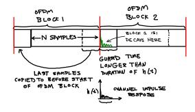
OFDM has become more popular than adaptive equalization because it is simpler to implement and more robust. This is partly because it is not necessary to estimate the channel to correct for ISI. OFDM is used by most modern ADSL, WLAN and 4G cellular standards.
