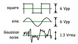
You will capture these waveforms with a digital oscilloscope. Then you will use Matlab to compute histograms that estimate the probability density functions of the waveforms. The histogram data will be imported into a spreadsheet that you will use to plot the histograms, compute the RMS powers from the probabilities and compare them to the powers measured using an RMS voltmeter and the oscilloscope's measurement function.
