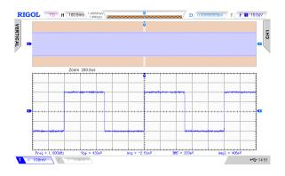
Use the DMM to measure the RMS value of the waveform. It should match the 'scope measurement value.
