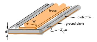
There are equations that accurately predict the characteristic impedance of microstrip transmission lines. We can also make a (very) rough estimate by assuming the trace forms a parallel-plate capacitor and using an approximate equation for the inductance of a trace over a ground plane.
