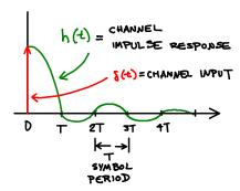
An example of an impulse response that meet this criteria is the sinc() function:
