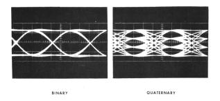
The vertical opening at the sampling time, called the "eye opening", represents the amount of ISI at the sampling point.
