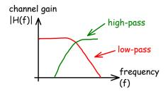
A band-pass channel is very common. A commonexample would be a transformer-coupled telephone line. Some band-pass channels result from attenuation by the channel but in other cases the band-pass nature of the channel intentional and is designed into the system to separate signals at different frequencies.
