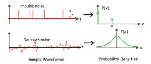
Signals that result from the sum of many small independent events have a probability distribution known as a Gaussian distribution. In communication systems this usually happens due to the sum of of voltages produced by the actions of very many individual photons, electrons or molecules.
