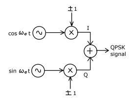
The equation for the modulated signal is:
