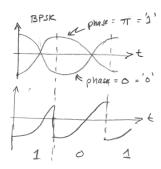
We can also vary the phase of the signal by other amounts. For example, we can use phase shifts of 0, 90, 180 and 270 degrees to transmit 4 different phases.
