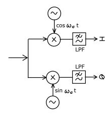
The receiver has to recover the phase of the carrier to accurately set the I and Q phases. This can be done, for example, by transmitting a preamble that has a known phase.
