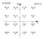
where each point is labelled with the bits that are transmitted if that symbol (a carrier with the given I and Q amplitudes) is transmitted. However we can transmit twice as much data: the real and imaginary components can be modulated independently.
