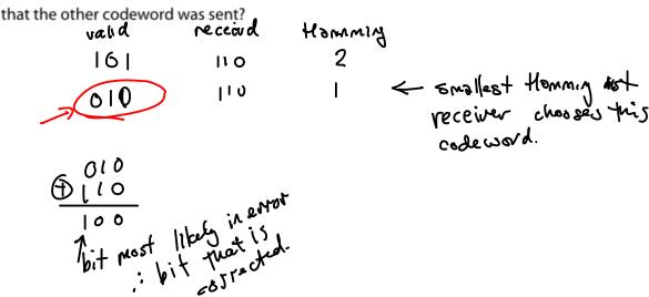
**Exercise 6**: What is the minimum distance for the code in the previous exercise? How many errors can be detected if you use this code? How many can be corrected? What are n, k, and the code rate (k/n)?
