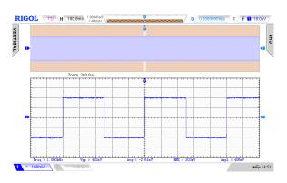
Use the DMM to measure the RMS value of the waveform. It should match the 'scope measurement value.
