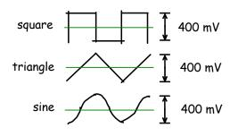
You will capture these waveforms with a digital oscilloscope. Then you will use Matlab to compute histograms that estimate the probability density functions of the waveforms. The histograms will be imported into a spreadsheet and you will use the spreadsheet to plot the probability distributions, compute the RMS powers from the distributions and compare them to the powers measured using an RMS voltmeter and the oscilloscope's measurement function.
