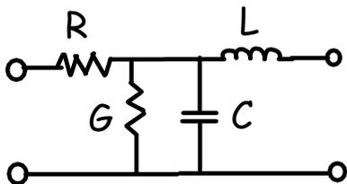
For the UTP cable the capacitance is specified as  $C = 15$  pF/ft or  $15 \times 3.28 = 49$  pF/m. The inductance was specified in the question as  $L = 525$  nH/m. The DC resistance (per conductor) is given as 9.38 Ohms/100m so the resistance in the lumped-element model is  $R = 2 \times 9.38/100 = 0.19$  Ohms/m.
