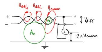
The area between the wires (Ad) is typically much smaller than the area between the wires and ground
