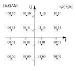
where each point is labelled with the bits that are transmitted if that symbol (a carrier with the given I and Q amplitudes) is transmitted.
