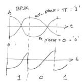
We can also vary the phase of the signal by other amounts. For example, we can use phase shifts of 0, 90, 180 and 270 degrees to transmit 4 different phases.
