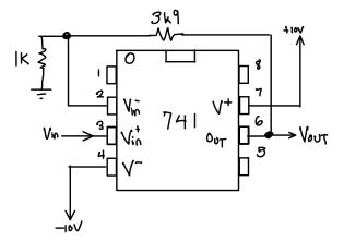
Build the amplifier circuit on your prototyping board using the components supplied in the lab.
