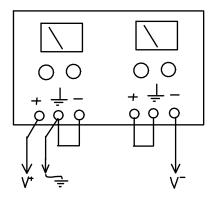
Double-check your circuit. Check it again. Set the power supply voltages before connecting them to your circuit. Make sure the voltages are not being limited by the current limiting controls.
