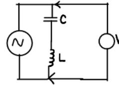
The inductance can be measured indirectly by measuring the resonant frequency of this LC circuit.
