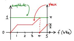
Will a 2 kHz sine-wave signal be distorted? How about a signal that contains both 1 kHz and a 2 kHz frequency components?
