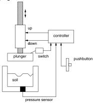
The device operates as follows: The operator puts soil in the container and presses the pushbutton. The controller moves the plunger down until the pressure indicator indicates that the pressure has reached a sufficiently high level. At this point the motor is shut off. When the operator pushes on the button again, the plunger is raised until it reaches the fully-retracted position.
