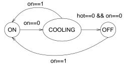
There are many different conventions for drawing state diagrams. For example, it's common to also show the values of the outputs on the state diagram. In the examples in this course we will describe the output values for each state separately.
