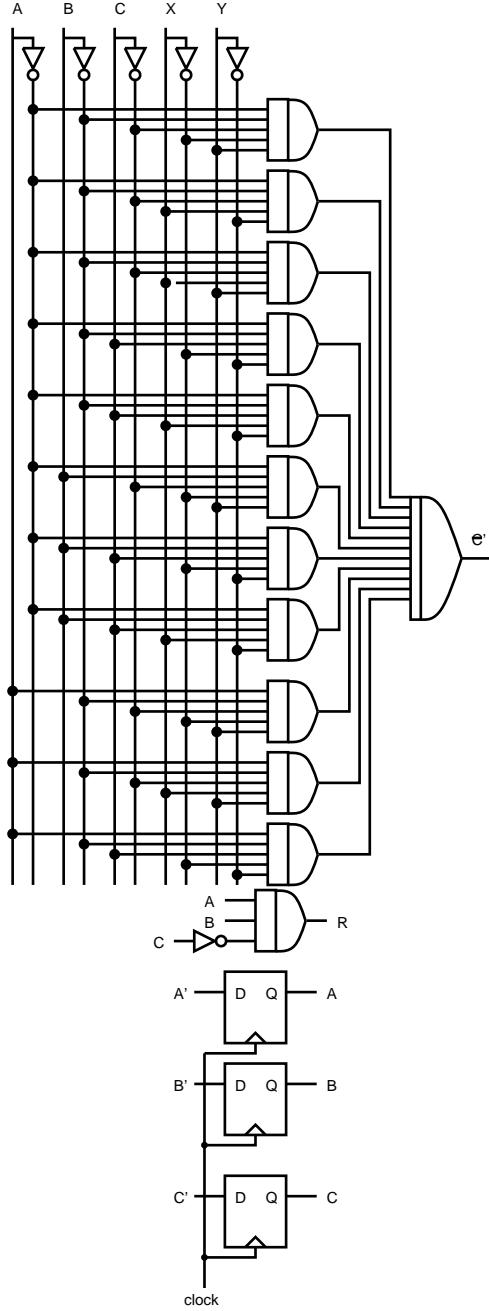
In this particular design the candy release signal will be high (equal to one) for one clock period (1 ms).
