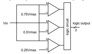
All of the digital outputs connected to reference voltages below the input signal will be true and all of the outputs with reference signals above the input signal level will be false. The output logic circuit converts these  $2^N - 1$  binary values into an N-bit number.
