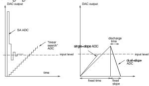
This method can be quite slow since sufficient conversion time must be allowed the counter must count up to  $2^N$ . However since this method is quite accurate it is often used in high precision (e.g. 16-bit) converters.
