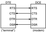
The second set of control signals are DTR (Data Terminal Ready) and DSR (Data Set Ready). These signals indicate that the DTE and DCE devices respectively are connected and operational (typically, simply that the power is turned on). Some modems can use DTR to force a reset and DSR as a replacement for CD (see below).
