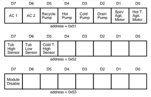
The 8 bits of the port at address 0x51 are connected to 8 output modules. The bits of an output module can be set by writing the appropriate bit pattern to the appropriate location.
