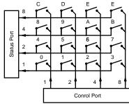
The keypad consists of 16 switches arranged in a square matrix. Each pushbutton controls a switch which can make a connection between a wire running horizontally and a wire runing vertically.
