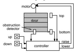
The controller has five inputs: two pushbuttons to request that the door be opened (up) or closed (down), two switches that indicate when the door is at the top or bottom of its range and a switch that indicates that the door has hit an obstruction. The controller has two outputs that control a motor: one to raise and one to lower the door.
