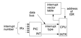
On the IBM AT and later models there are more than 8 interrupt sources and there are two PICs. The slave PIC supports an additional 8 interrupt inputs and requests an interrupt from the master PIC as if it were an interrupting peripheral on IR2.
