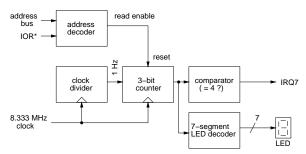
The device has a 3-bit counter that is incremented once per second. A 1 Hz signal is generated using a clock divider as in Lab 3. The count is displayed on a 7-segment LED display as in Lab 2. The port generates an interrupt by asserting the PC-104 bus interrupt request number 7 (IRQ 7) when the counter value reaches 4. This bus signal is connected to IR7 on the SBC's 8259 PIC.
