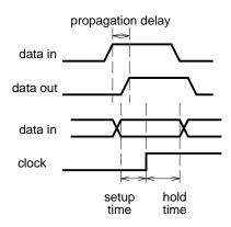
The most common guaranteed response is the *propagation delay* which is the maximum delay between a change in the input and the correct value appearing at the output. A similar guaranteed response during a memory device read cycle is the *access time*. This is typically measured from the address, chipselect, or output-enable signals changing to when the data outputs become valid.
