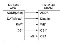
The microprocessor's data strobe (DS\*) signal drives the RAM's chip select (CS1\*). The RAM's write enable (WE\*) is driven by the CPU's read/write signal (R/W\*). The RAM's address and data buses are connected to the corresponding CPU buses.
