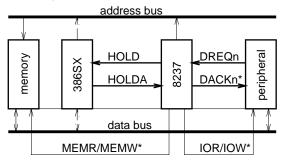
The DMA controller uses hold request (HOLD) and hold acknowledge (HOLDA) signals to ask the CPU to stop driving the address, data and control buses so that the DMA controller can drive them to carry out a transfer.
