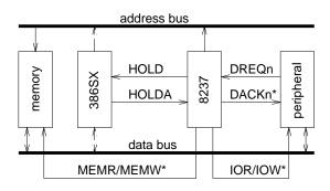
The DMA controller uses the CPU's hold request (HOLD) and hold acknowledge (HOLDA) signals to ask the CPU to stop driving the address, data and control buses so that the DMA controller can use them to carry out a data transfer.
