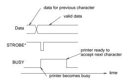
There are additional handshaking lines to control various printer features (e.g. auto line feed) and to indicate various printer status conditions (e.g. out of paper).
