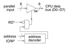
The value read by the CPU will be the value on the input at the time that the port is read.
