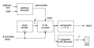
The device has a 3-bit counter that is incremented once per second. The 1 Hz clock is generated using a clock divider as in Lab 3. The count is displayed on a 7-segment LED display as in Lab 2. The port generates an interrupt by asserting the PC-104 bus interrupt request number 7 (IRQ 7) when the counter value reaches 4. This bus signal is connected to IR7 on an 8259 PIC.
