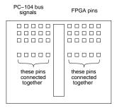
There are two interconnect boards. The left interconnect board is used to connect the PC-104 data and address bus and the board on the right is used to connect the memory/I/O read/write strobes and the interrupt request lines.
