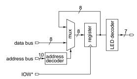
The inputs are the LS 10 bits of the address bus<sup>1</sup>, the 8 bits of the data bus, and the IOW\* write strobe.
