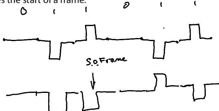
**Exercise 2:** Preambles such as this allow multiple transmission formats to be used in a backwards-compatible way. What might be some disadvantages of using such a preamble? Hint: to be decoded by old ("legacy") devices the preamble must be transmitted at the lowest possible data rate. This can be 100 times slower than the fastest devices.
