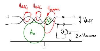
The two conductors of the twisted pair are next to each other and the area between the wires  $(A_d)$  is much smaller than the area between the wires and ground  $(A_c)$ . This will result in a smaller voltage being induced on the differential signal. In addition, the voltages induced on the twisted pair by the magnetic field (the parts of the field  $H_{diff+}$  and  $H_{diff-}$ ) will cancel out due to the twisting.
