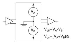
A differential transmitter encodes data as the voltage difference between its two outputs. For example,  $V_A = +5 \, \text{V}$  and  $V_B = 0 \, \text{V}$  for a logical '1' and  $V_A = 0 \, \text{V}$  and  $V_B = +5 \, \text{V}$  for a logical '0'. The differential receiver finds the differential volatage by subtracting the two voltages (resulting in differential volages of +5 V and -5 V for this example).
