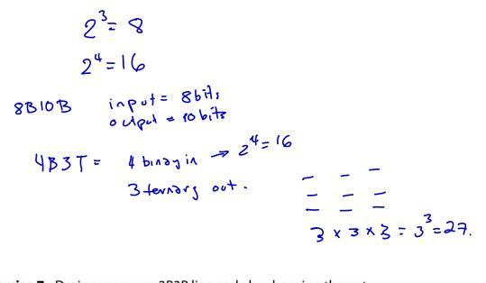
**Exercise 7**: Design your own 2B3B line code by choosing the output waveforms that have the lowest average DC value and giving preference to those that start and end at different levels (assume bipolar signalling).
