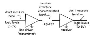
The ICL-232 includes two line drivers (transmitters) and two receivers. You can test either one of the two transmitters and either one of the two receivers.
