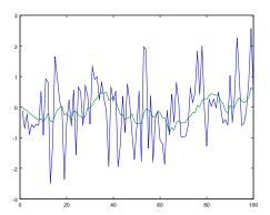
It's clear that the power of the low-pass filtered version is significantly less than the unfiltered signal.
