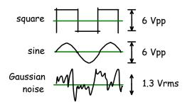
You will capture these waveforms with a digital oscilloscope. Then you will use Octave<sup>1</sup> to compute histograms that estimate the probability density functions of the waveforms. The histogram data will be imported into a spreadsheet that you will use to plot the histograms, compute the RMS powers from the probabilities and compare them to the powers mea-
