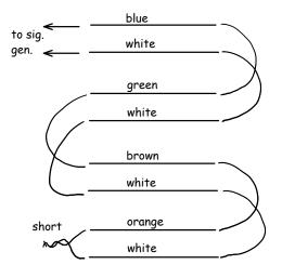
increase the frequency until the signal level is minimum. If you have one of the longer lengths of cable you might see multiple nulls; use the first (lowest frequency) null to compute the length. Note that at low frequencies the shorted transmission line also acts as a short circuit.
