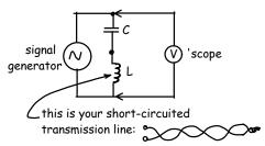
The inductance can be measured indirectly by measuring the resonant frequency of this LC circuit.
