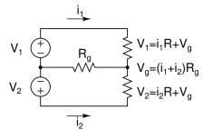
These effects can be particularly severe when the shared ground circuit is used as the return path for a power supply.
