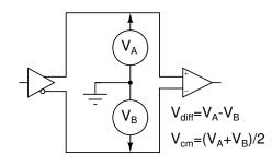
A differential transmitter encodes data as the voltage difference between its two outputs. For example,  $V_A = +5$  V and  $V_B = 0$  V for a logical '1' and  $V_A = 0$  V and  $V_B = +5$  V for a logical '0'. The differential receiver finds the differential voltage by subtracting the two voltages (resulting in differential voltages of +5 V and -5 V for this example).
