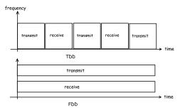
Many cellular systems use both TDD and FDD. TDD avoids the need for duplexers and FDD reduces the potential for transmissions to interfere with nearby receivers.
