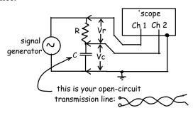
There is no actual capacitor used for this measurement. In the schematic above the capacitor is actually the transmission line. One side of the twisted pair goes to ground and the other side to the bottom of the resistor. The twisted pair you are measuring is open-circuited at the other end and so in effect you are forming a capacitor from two pieces of wire that run parallel to each other for a meter or two. This is the capacitor in the schematic and the capacitance that you will measure.
