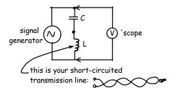
The inductance can be measured indirectly by measuring the resonant frequency of this LC circuit.
