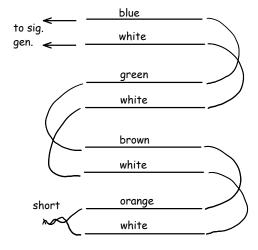
• increase the frequency until the signal level is minimum. If you have one of the longer lengths of cable you might see multiple nulls; use the first (lowest frequency) null to compute the length. Note that at low frequencies the shorted transmission line also acts as a short circuit.
