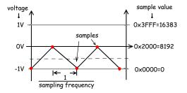
The samples values are stored in binary format in *little-endian* byte order. The the contents of the file for the waveform above would be as shown in the following hex dump:
